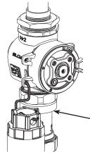
NOTE: If desired, orange flow adjustment tool can be attached to valve assembly using supplied mounting hanger
