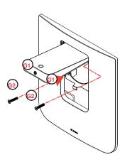
Choose one of three Plunger screws and nut provided and thread into plunger. If Plunger starts rotating, STOP. This means the screw has reached the bottom of the hole and overtightening the screw will cause damage to the plunger. Try the next shorter screw included with the product to finish adjustment.
