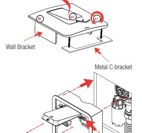
Mount wall bracket to wall, tilting to insert metal C-bracket through wall opening.
